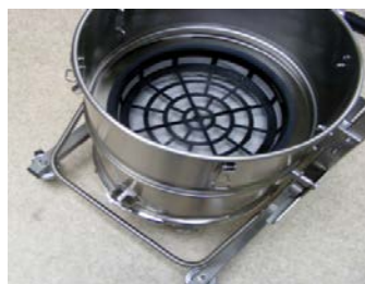
Interior view with filter stage 2
