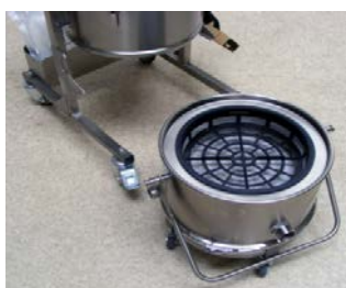
Dirt tank with filter stage 2
