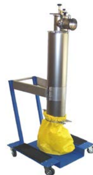
Preseparator for fine dust with bag
