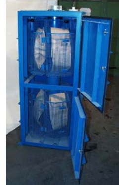
Cabinet for dust collection with multiple paper bags
