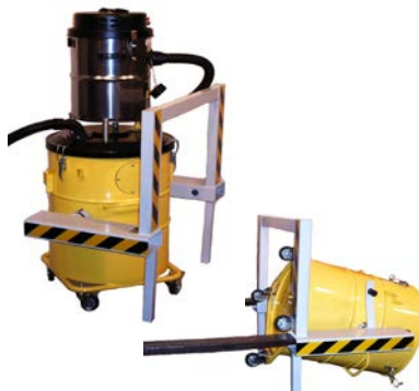
Preseparator to use with a fork lift
