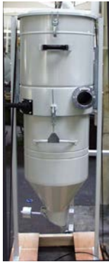
Preseparator with filter
