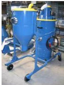
Preseparator to use with a fork lift
