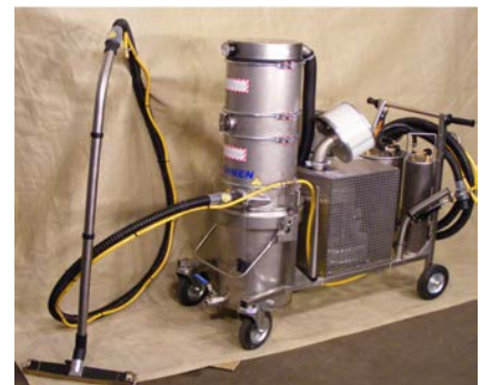
DGS 50 EX with spraying system and additional filter
