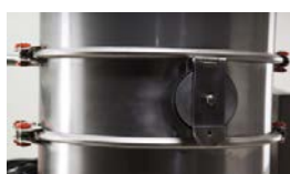
FDR Filter cleaning system
